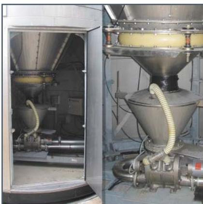
◀ Through the silo door there is easy access to emptying and weighing equipment.
