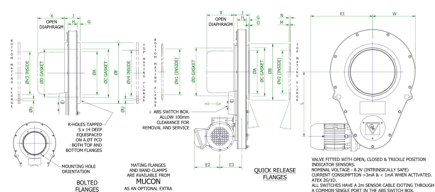
**OPERATION BY 0.25kW** 2-POLE, IP66 INDUCTION MOTOR. SUITABLE FOR: 230/400V - 3ph - 50Hz SUPPLY.
