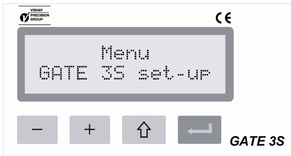
Figure 4. Before parameter editing can start, GATE 3S must be switched over to Set-up mode, indicated by this menu.
