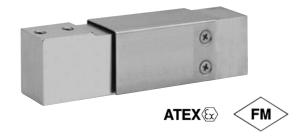
bench and counting scales. For wash-down protection an optional IP65 encapsulation protection is available. Constructed from stainless steel this high accuracy load cell is approved to Factory Mutual and other stringent approval standards.
