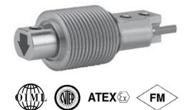
The low profile, high accuracy and sealing makes this load cell highly suitable for applications such as low profile platforms, weighing and packing machines, conversion of mechanical scales and variety of other applications where sealed cells are required. For hazardous environments this load cell is available with EEx ia IIC T6 level of approval as an option.
