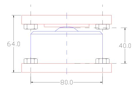
NB: The height of 64 mm is inclusive the isolation mount above and under the load cell.
